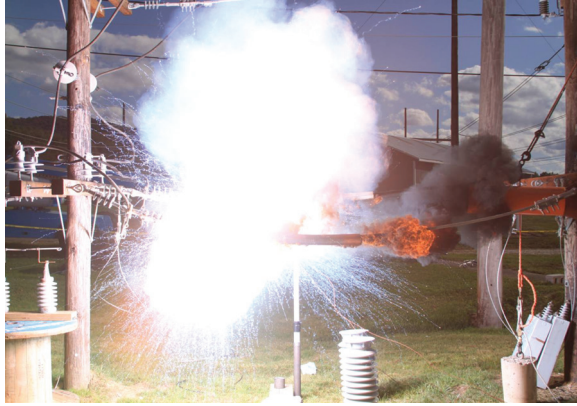
Figure 2.20 Burndown test with line hose. (Electric Power Research Institute. 1017839, Distribution Conductor Burndown Test Results. Copyright 2009. Reprinted with permission.)
