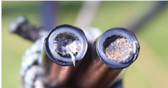
Figure 2.19 Example of burndown damage on covered 336-kcmil AL conductors. (Electric Power Research Institute. 1017839, Distribution Conductor Burndown Test Results. Copyright 2009. Reprinted with permission.)
