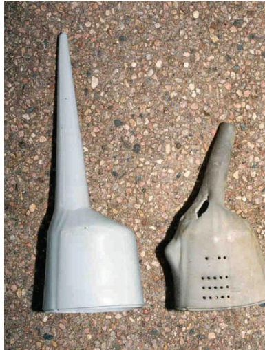
Figure 3.21 Example of a deteriorated animal guard compared to a new animal guard. (From EPRI TE-114915, Mitigation of Animal-Caused Outages for Distribution Lines and Substations , Electric Power Research Institute, Palo Alto, CA, 1999. Copyright 1999. Reprinted with permission.)
