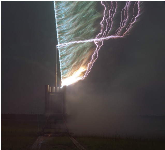
Figure 13.24 Lightning flash triggered by a rocket trailing a wire. (From Electric Power Research Institute. Copyright © 1993. Reprinted with permission.)
